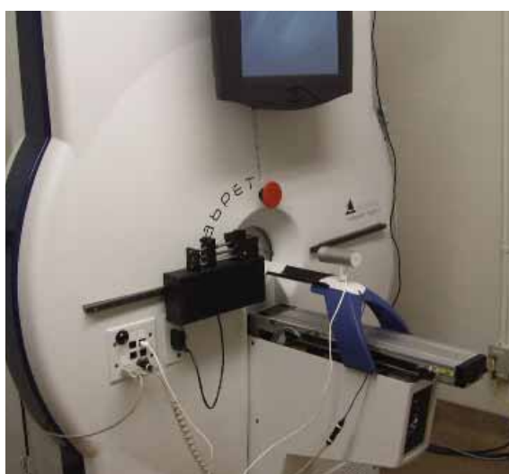
UOHI's new MicroPET measures blood flow to the heart and the chemistry of the heart muscle in a mouse heart that is about the size of a pencil eraser.
